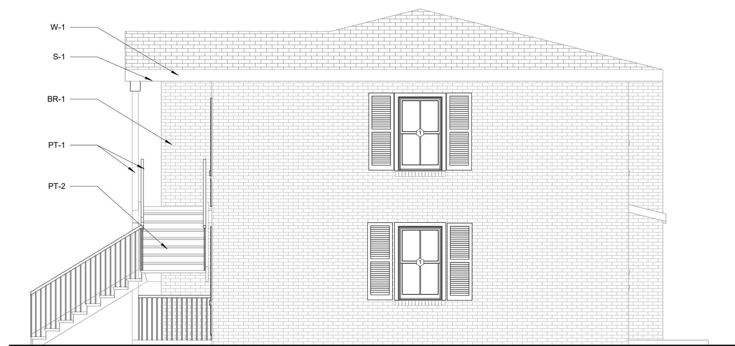
4 E-1A NEW CONSTRUCTION SIDES 1/4" = 1'-0"
