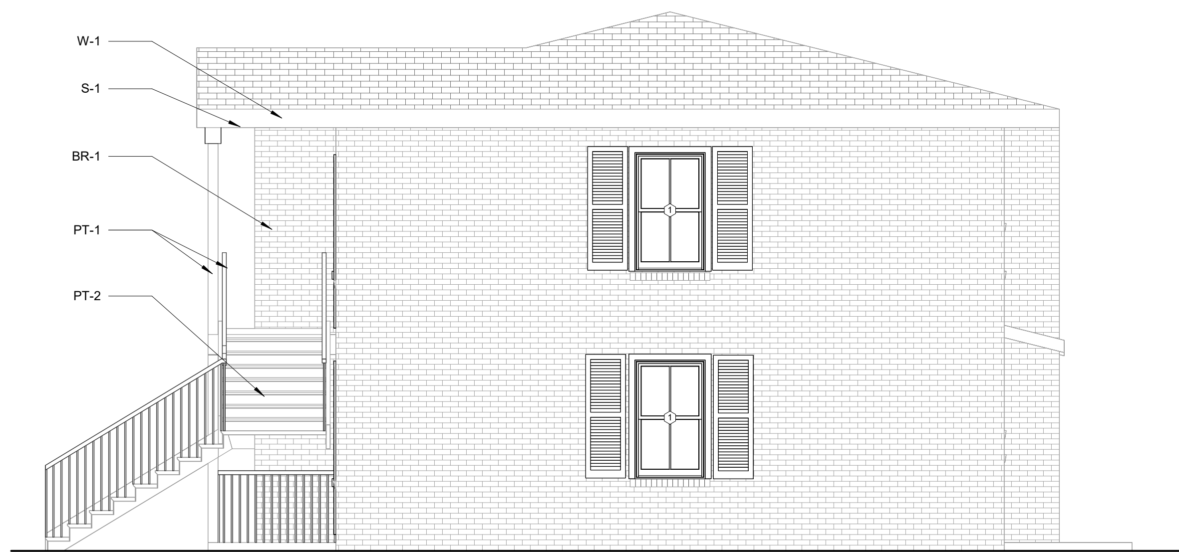
4 E-1A NEW CONSTRUCTION SIDES 1/4" = 1'-0"
