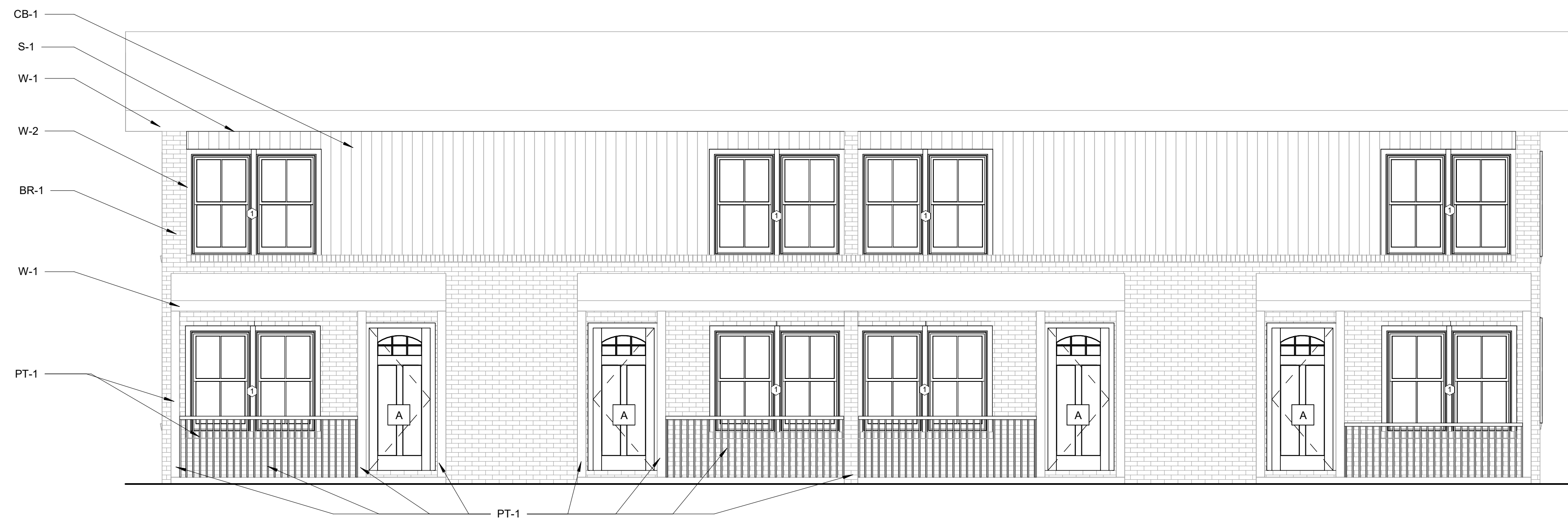
1 B-4A NEW CONSTRUCTION FRONT 1/4" = 1'-0"
