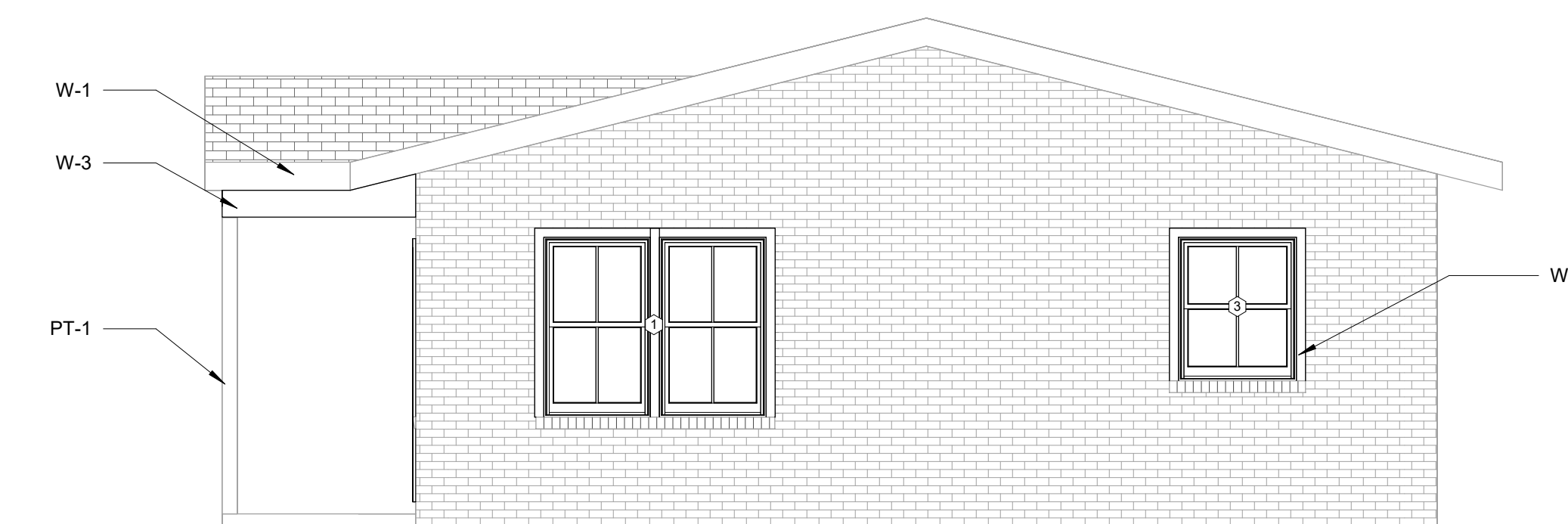
5 D-2B/D-2C NEW CONSTRUCTION SIDES 1/4" = 1'-0"
